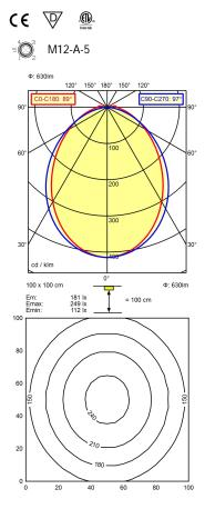
light source LED work equipment without connected load 22-26 V, DC env. 5 W power consumption luminous flux approx. 630 lm luminous efficiency approx. 126 lm/W light type/-color cold white colour temperatur approx. 5.000 K CRI > 80 color rendering index light distribution direct beam angle 89° / 97° chromaticity tolerance LED < 4 SDCM glare control screen system of protection IP 54
